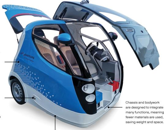
Compressed air tanks mean no chemical batteries, and stored energy remains available without deterioration, with each tank having an estimated lifespan of 20,000 cycles.
